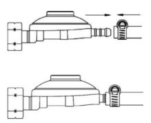
Connect the gas regulator to the cylinder of gas by turning the knob clockwise until it stops. It must then be further tightened using a spanner. Make sure that the tube is not twisted.
